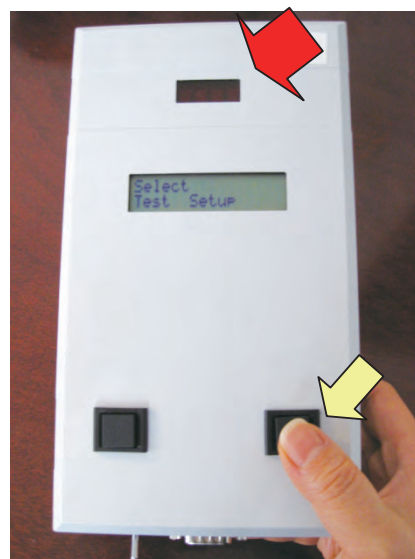
Figure 2 Psychomotor Vigilance Task. When a light flashes on the upper screen (flashes were presented at randomly defined intervals), the subject presses the button at the bottom.
